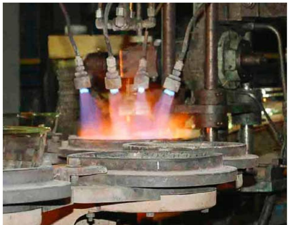
Energy intensive reheat burners keep process equipment hot to avoid inducing a temperature shock in the glassware.
